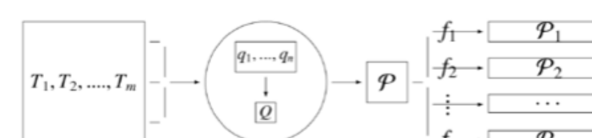
Fig. 8. The CheetahDB concurrent query processing system model. T_1, T_2, \dots, T_m are input tables, p_1, p_2, \dots, p_n are output tables for the n queries
